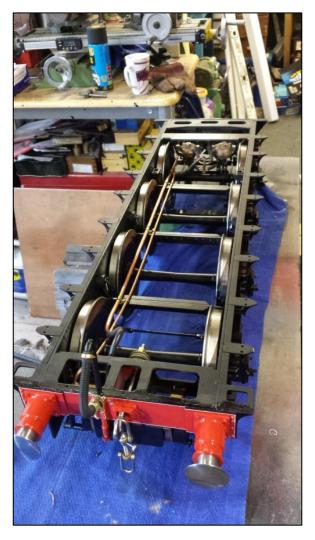
The chassis fully is painted although has a few bits of the lining to finish, most of it is there. The tender as with the locomotive is vacuum braked, both having two vacuum cylinders, these are all finished and tested. it's a shame that you can't add video to а newsletter...©
