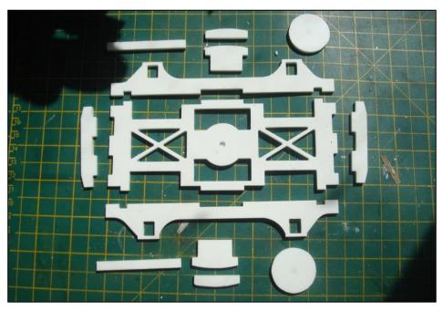
I have been fairly busy myself; these 2 photos' show the CNC cut parts (3mm HIP's) for my Pullman bogies, details on the finished bogie are in cast white metal, wheels are G1MRA.
